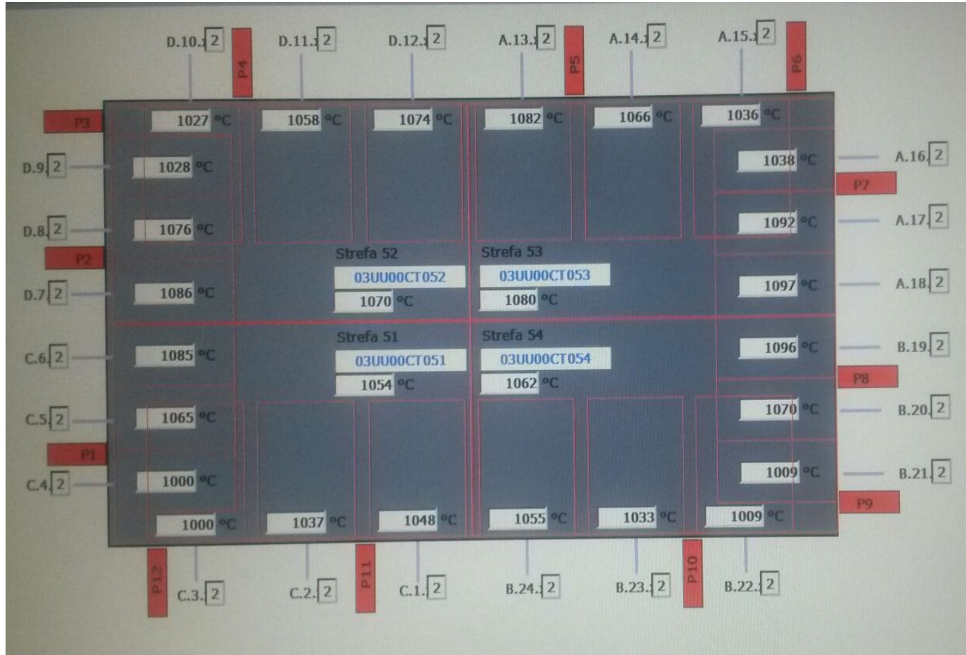
Temperature Indication at the Injectors
