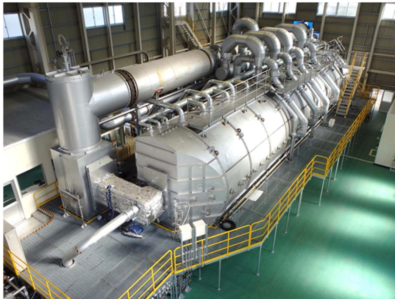
Combustion test furnace (4 t/h)
