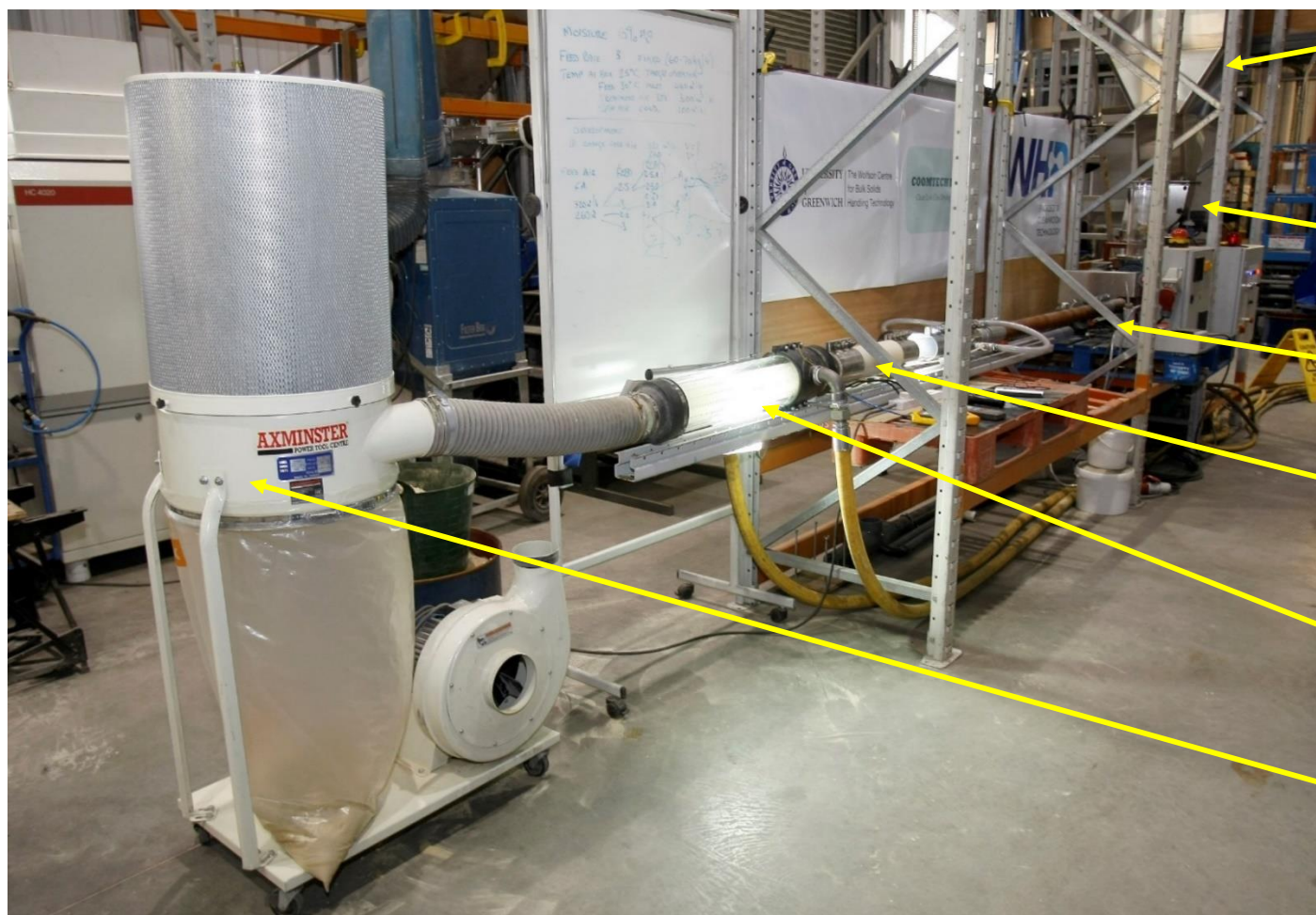
Coomtech Single Drying Zone Pilot Pre Industrialisation Configured in Perspex
