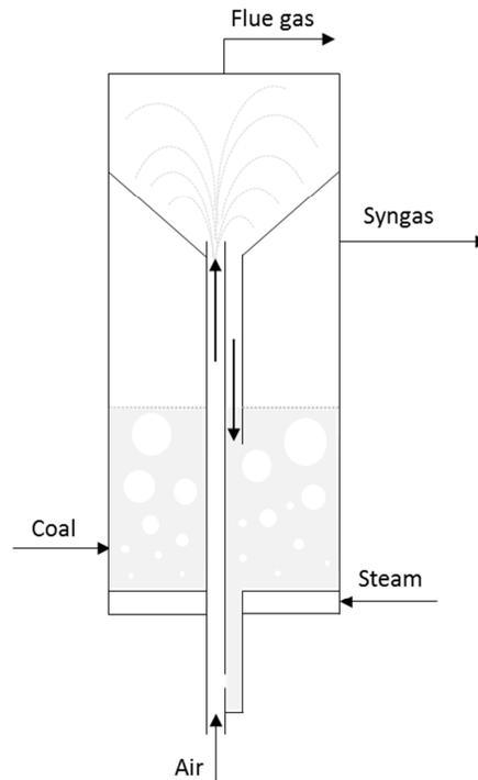
**Fig. 3: Schematic layout of the i-MILENA gasification concept**
