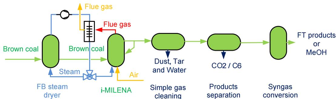
Fig. 7: (High ash) low rank gasification for synthesis of fuels & chemicals (100 – 1000 MW<sub>th</sub>).
