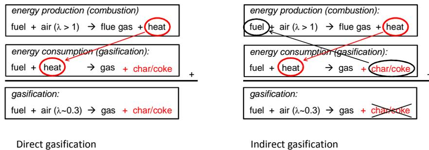
**Fig. 2: Direct gasification (left) leaves a solid combustible residue called char or coke, whereas indirect gasification (right) uses this as an energy source within the process, leading to a much higher overall efficiency.**
