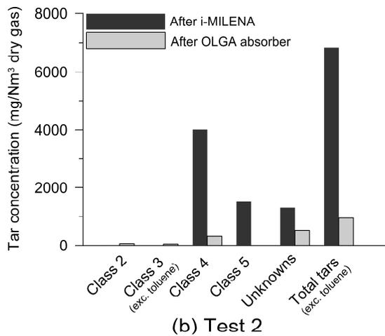
Fig. 6: Performance of OLGA tar removal system during i-MILENA tests with Indian high-ash coal.
