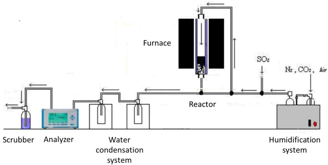
Figure 1. Experimental scheme of the dry desulfurization experiments.
