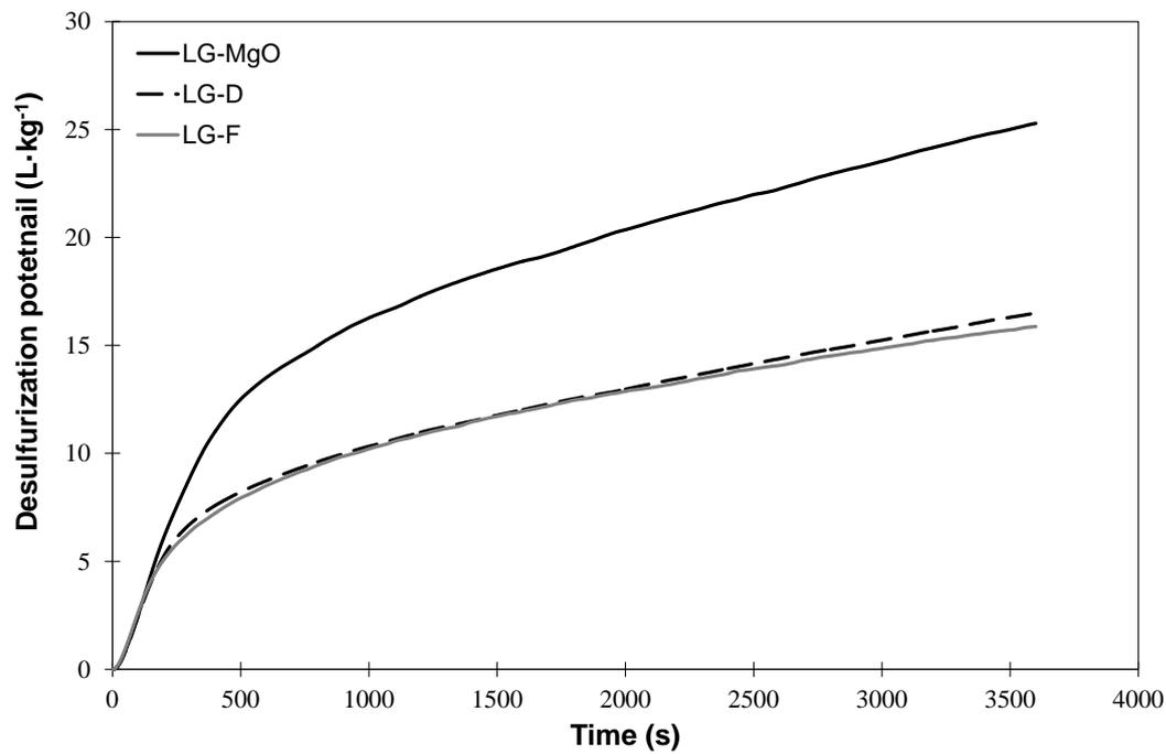
Figure 6. Desulfurization potential (volume of  $\text{SO}_2$  absorbed per mass of by-product) of 1 g of each of the by-products ( $\text{L}\cdot\text{kg}^{-1}$ ).
