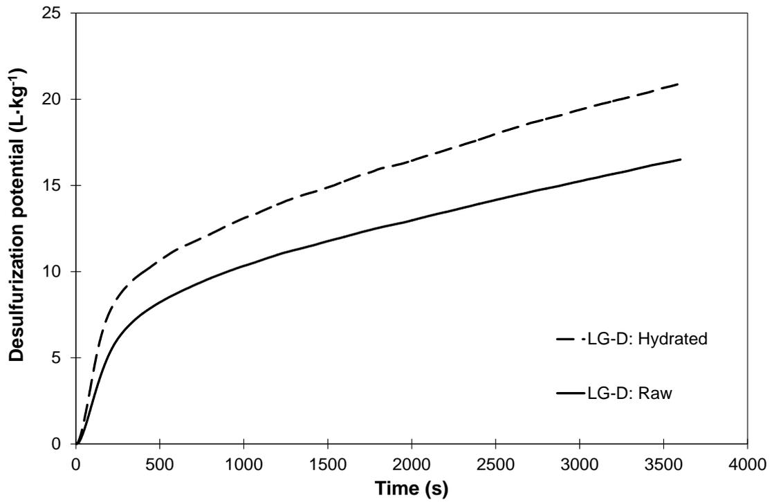
Figure 9. Desulfurization potential (L·kg<sup>-1</sup>) of raw and hydrated LG-D.
