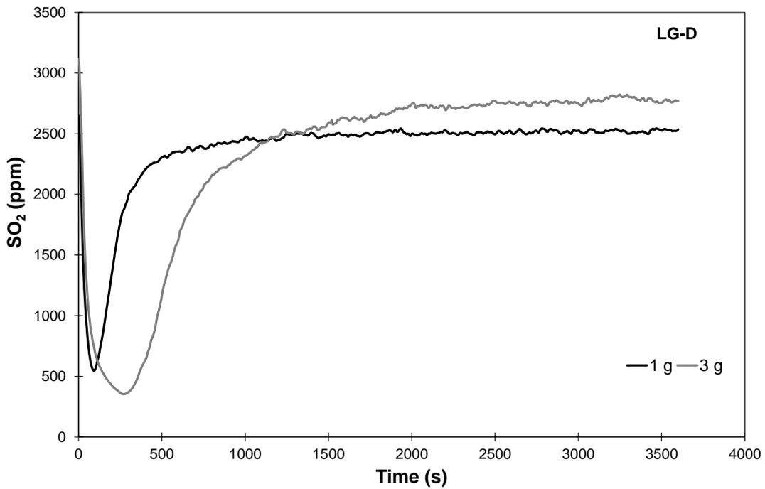
Figure 4. Concentration of SO<sub>2</sub> at the outlet (ppm) as a function of time (s) for raw LG-D. Effect of mass sample.
