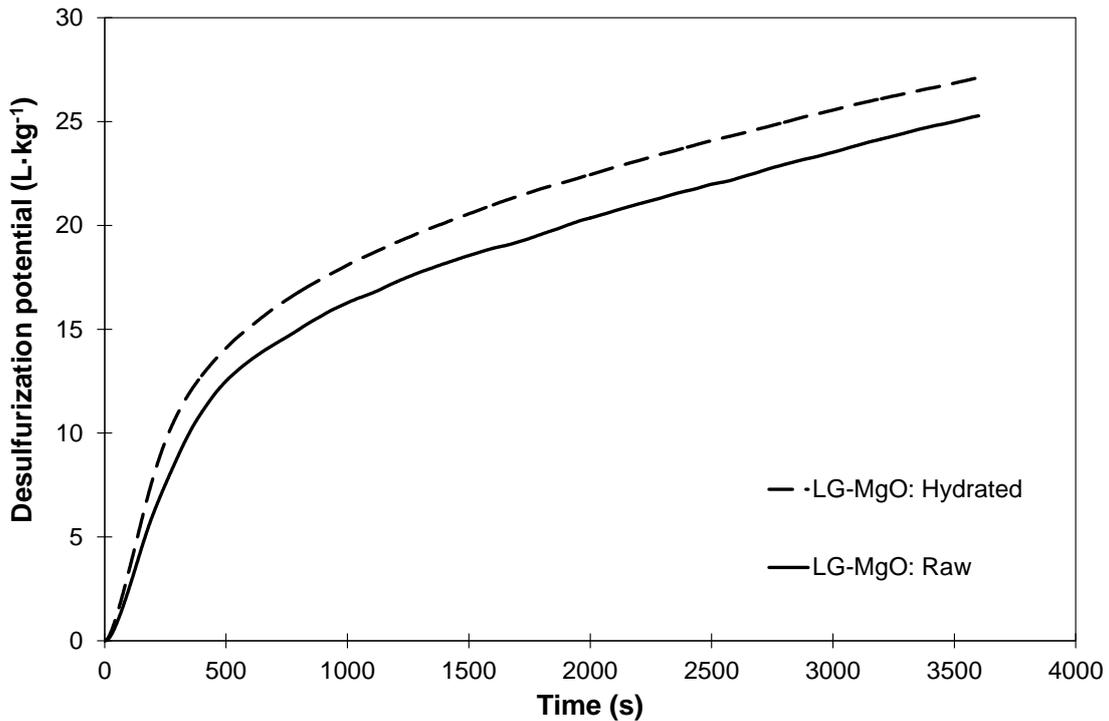
Figure 8. Desulfurization potential (L·kg<sup>-1</sup>) of raw and hydrated LG-MgO.
