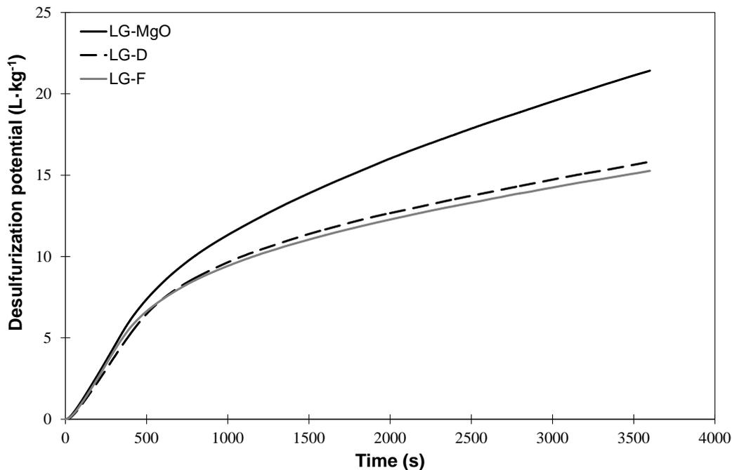
Figure 7. Desulfurization potential (volume of  $\text{SO}_2$  absorbed per mass of by-product) of 3 g of each of the by-products ( $\text{L}\cdot\text{kg}^{-1}$ ).
