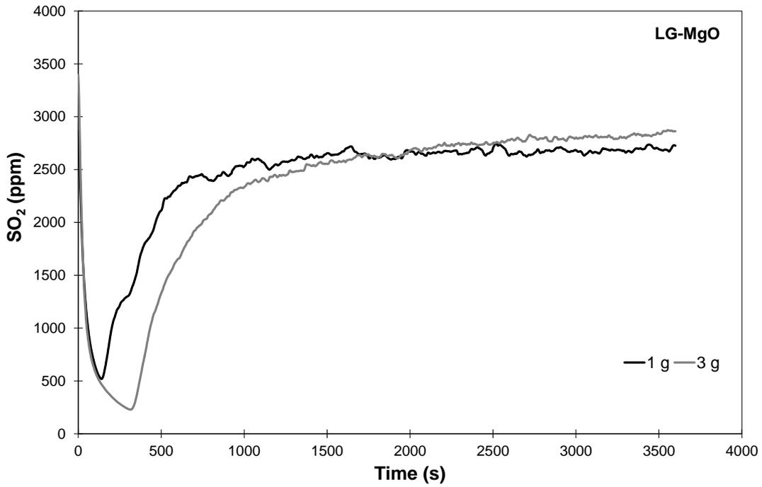
Figure 3. Concentration of SO<sub>2</sub> at the outlet (ppm) as a function of time (s) for raw LG-MgO. Effect of mass sample.
