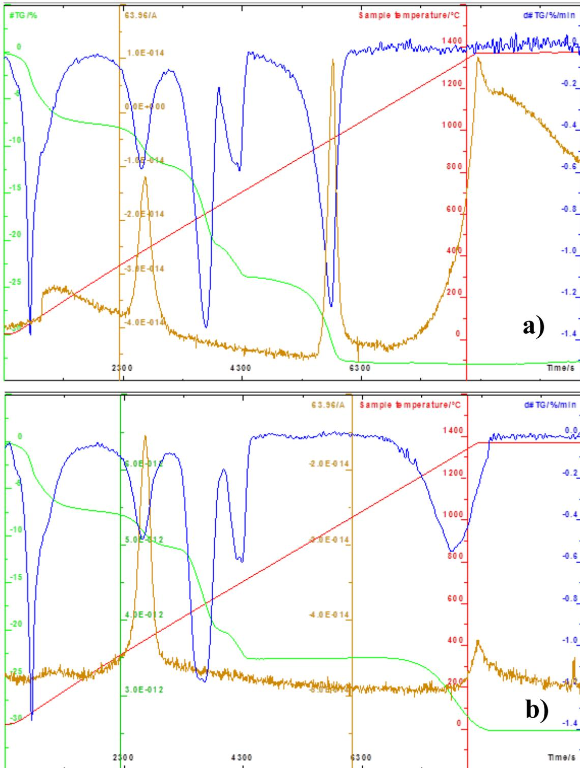
Figure 10. TG, DTG and MS curve ( $\text{M}^+ 64$ , corresponding to  $\text{SO}_2$ ) of raw LG-MgO after desulfurization using  $\text{N}_2$  as the carrier gas (10a) and synthetic air (10b).
