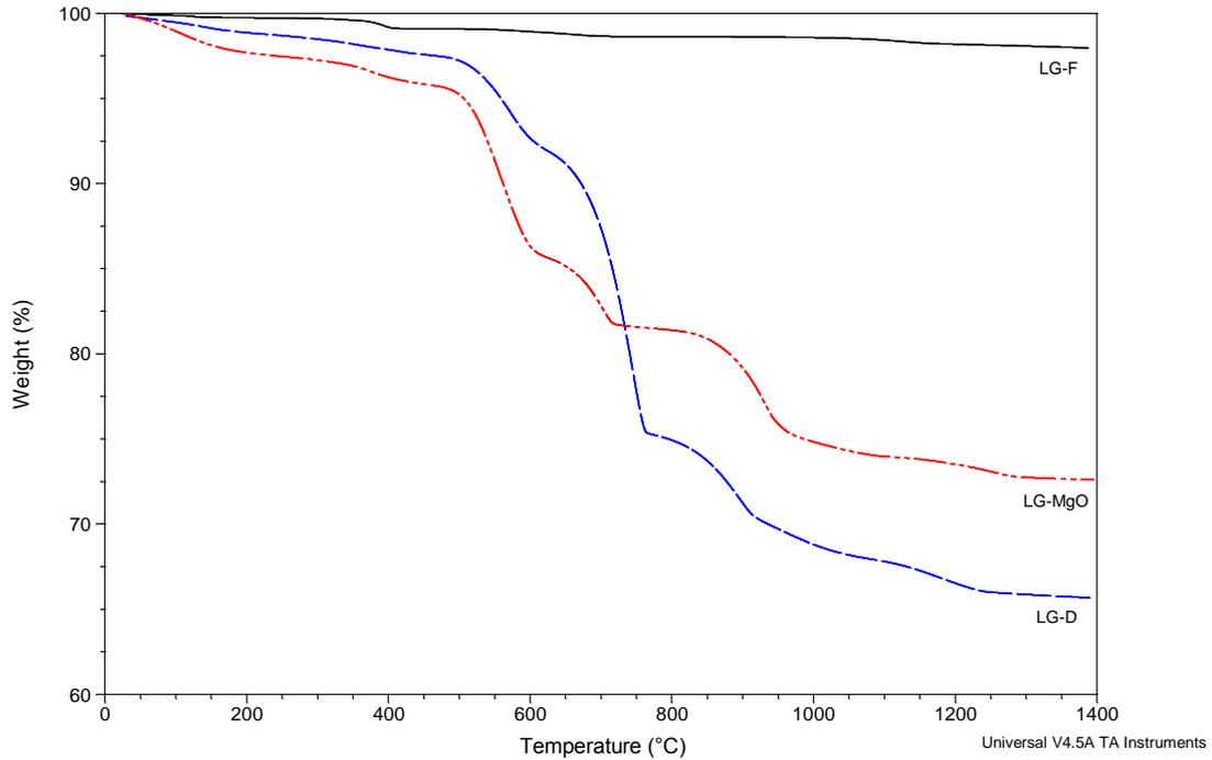
Figure 2. TGA of the raw by-products (LG-MgO, LG-D and LG-F).
