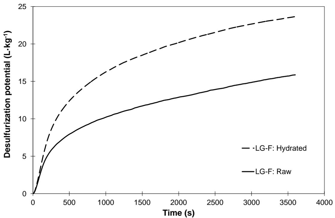
Figure 10. Desulfurization potential (L·kg<sup>-1</sup>) of raw and hydrated LG-F.
