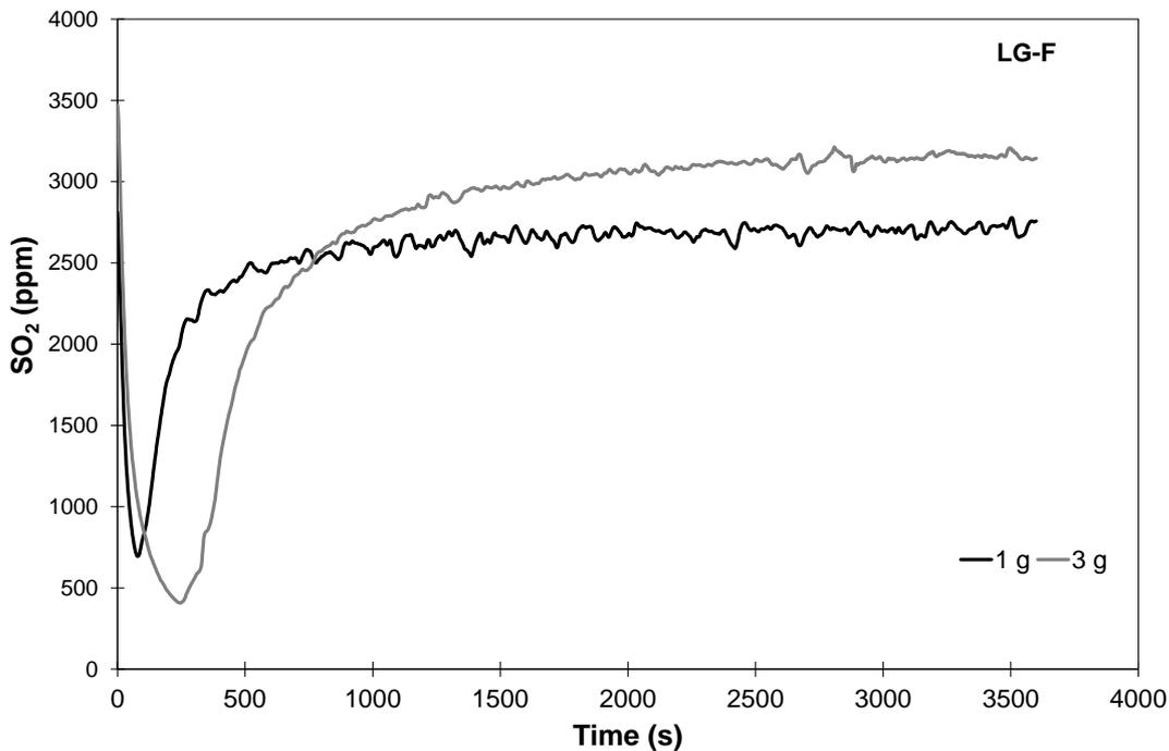
Figure 5. Concentration of SO<sub>2</sub> at the outlet (ppm) as a function of time (s) for raw LG-F. Effect of mass sample
