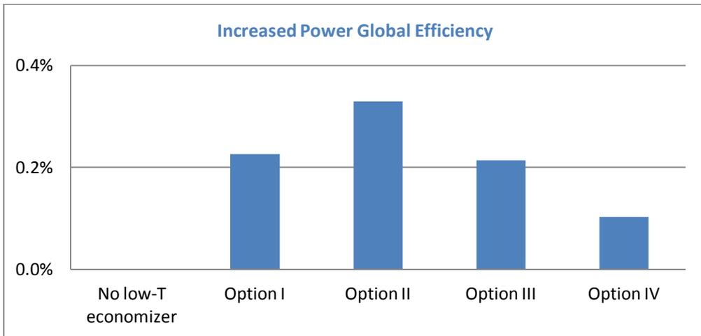
Figure 4 Power plant efficiency increase (% points) in operation case with Option I, II, III & IV<sup>2</sup>
