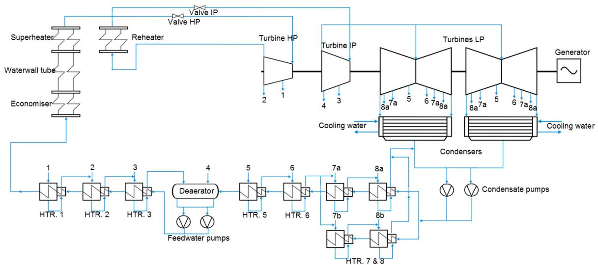
**Figure 1 Flowsheet of the 600MWe coal-based power plant**
