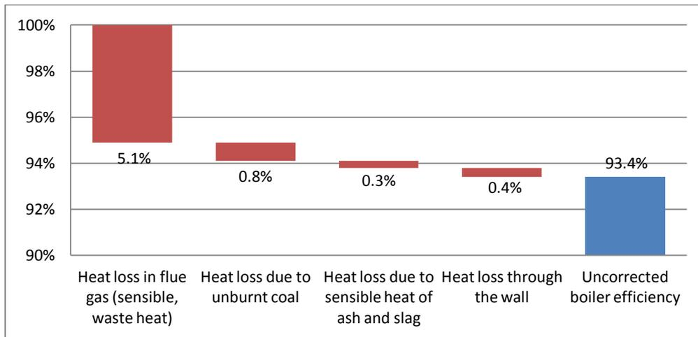
Figure 5 Boiler efficiency in operation case after adding Option I LTE
