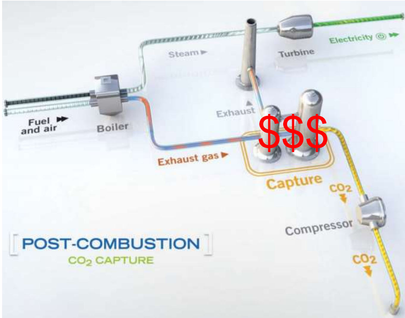
Fig. 1. Conventional post-combustion CO 2 capture using absorption process.
